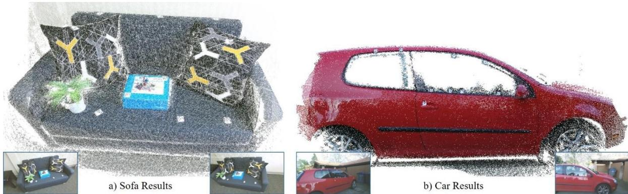
**Figure 3: Initial HawkEye Pipeline Results.** Initial experiments investigated the effectiveness of the HawkEye reconstruction pipeline using two datasets: an indoor scene of a sofa (8 snapshots) and an outdoor scene of the side of a vehicle (6 snapshots). The pipeline clearly aligns the scanner data to produce visually accurate results.
