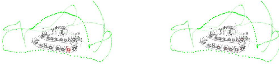
Figure 7: Impact of the spatial distribution of 3D scene points on pose estimation. For this experiment, 50 ground truth points are used to solve for camera pose. These points are arranged in two spatial distributions: a small cluster on the object (left) and a random distribution across the object (right). Accuracy of the camera pose is the same for each point distribution. The results for the bradley dataset are shown here: camera positions are displayed in green, the points selected for pose estimation are shown in red, and remaining points from the model are shown in dark grey.
