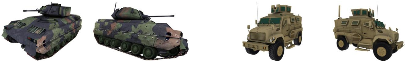
Figure 4: Synthetic datasets used to analyze camera pose estimation. These 3D models correspond to real assets, but can be rendered using known parameters, offering more control over the corresponding experimental results. Ground truth feature tracks are generated from the 3D object data. Two images from the bradley sequence are shown at left, while two images from the maxxpro sequence are shown at right. Both datasets are provided by SURVICE Engineering Company.
